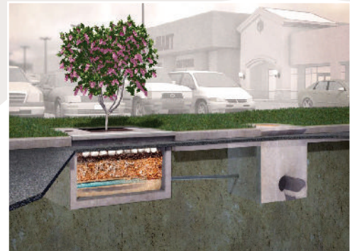
Standard Filterra System showing curb-inlet opening.
